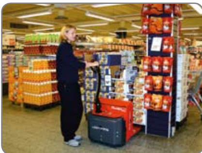
Panther Mini (capacity 1400 kg) is recommended for easy pallet transport, e.g. in super markets and in stock areas.
